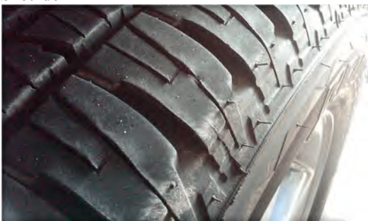
Figure 2: Tire Shoulder View Example 1 - "NORMAL" Tire "Feathering" Wear on the Shoulder
