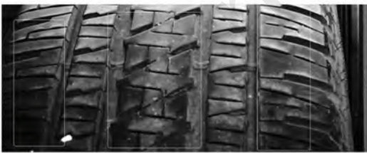
Figure 2: Tire Shoulder View Example 1 - "NORMAL" Tire "Feathering" Wear on the Shoulder
